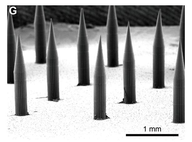
A close-up microscope image of the microneedle array, which could deliver quantum dots into skin. Credit: K.J. McHugh et al. *Science Translational Medicine* (2019)
